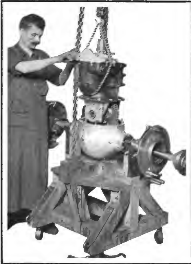
The axles are placed in the rear axle housing, and when the front end assembly has been fitted to the gearbox the workman assembles the gearbox and rear axle units
